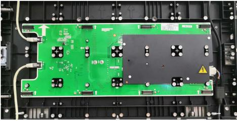
A photograph showing the board being reinstalled into the cabinet. The board is now secured with screws and the cables and power cords are reconnected. The yellow warning triangle is still visible.                                                                                                     | Replace a new board and fix it to the cabinet with screws. Then connect cables and power cords, and install modules back. |
