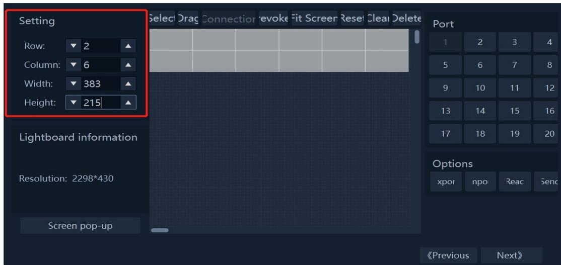
Step 3: Set the Ethernet port for cabinet and connection relationship, and click Send to send the cabinet set parameters
