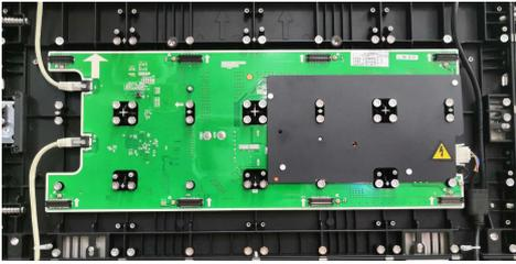
A photograph showing the green 2-in-1 board installed inside a black cabinet. The board is populated with various components, including capacitors and integrated circuits. A yellow warning triangle is visible on the right side of the board.                                                            | Find location of fault cabinet and remove all modules.                                                                    |
